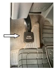
The emergency brake can be activated by pressing the emergency brake pedal on the floorboard or lifting the emergency brake lever between the seats depending upon how your car is designed.
