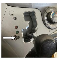
To shift from park to these other positions requires that the brake pedal be depressed. Note, also, that you should not force your car to go immediately from a forward to reverse direction of travel without first coming to a complete stop. We'll discuss these processes in greater detail later when we begin our exploration of basic driving maneuvers.
