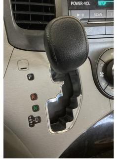
When the shift lever is in the P, or park, position, the wheels of the car are unable to move in any direction. The wheels are locked and this is the condition your car must always be left in after you're finished driving. Note in the photo here how this car is in park.
